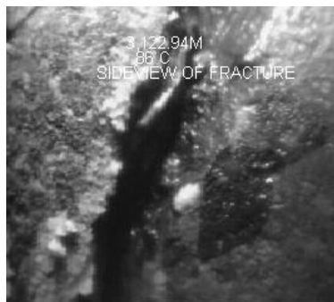
The ViewMax clearly identifies a fracture in the conglomerate of this open hole horizontal well
