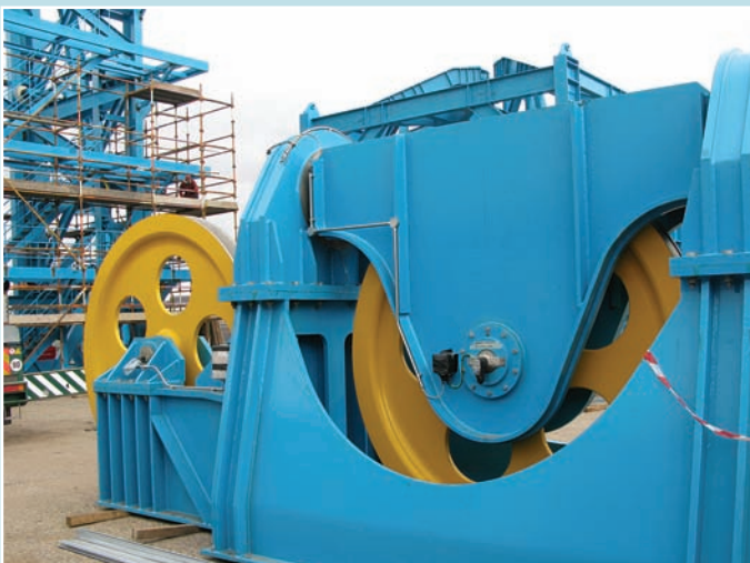
The top sheave of the handling tower
